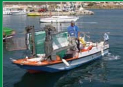
FCC uses 59 Marnett boats designed specifically for collecting floating and semi-submerged debris, seaweed and jellyfish in bathing areas.
